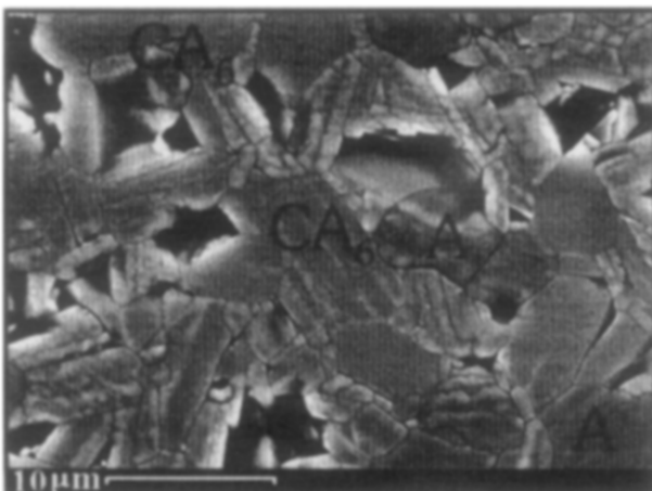
Fig. 9. Microstructure of compositions with low Fe_2O_3 content at very high temperatures.
